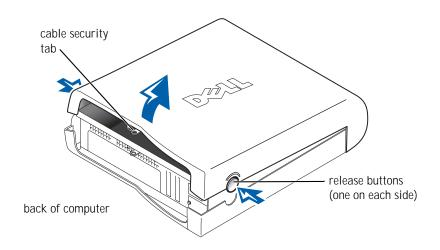
**HINT**: Make sure that the computer is oriented with the cable security tab on top, as shown in the illustration.
